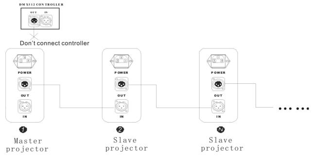
NB : in order to reduce signal errors, think of using a plug a the end of your DMX link.
